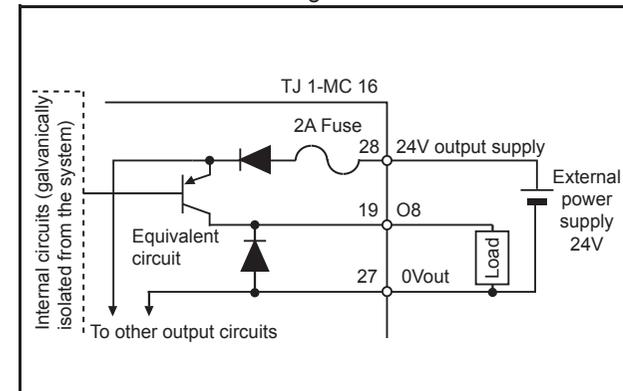
Maximum response times of 250  $\mu$ s on and 350  $\mu$ s off (for servo periods of 0.5 ms or 1.0 ms) or 500  $\mu$ s on and 600  $\mu$ s off (for a servo period of 2.0 ms) are achieved between a change in the OP parameter and a corresponding change in the digital output circuit.
