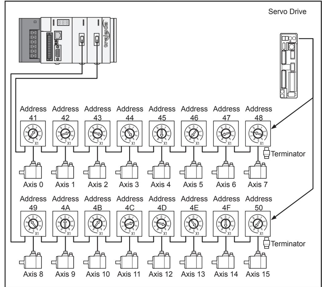
The MECHATROLINK-II Units can control different combinations of axes, Inverters and I/O units.
