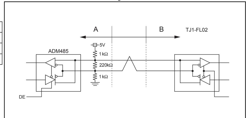
The table below and the figure give an example of how to connect the Tamagawa TS5667N420 encoder to the TJ1-FL02.
