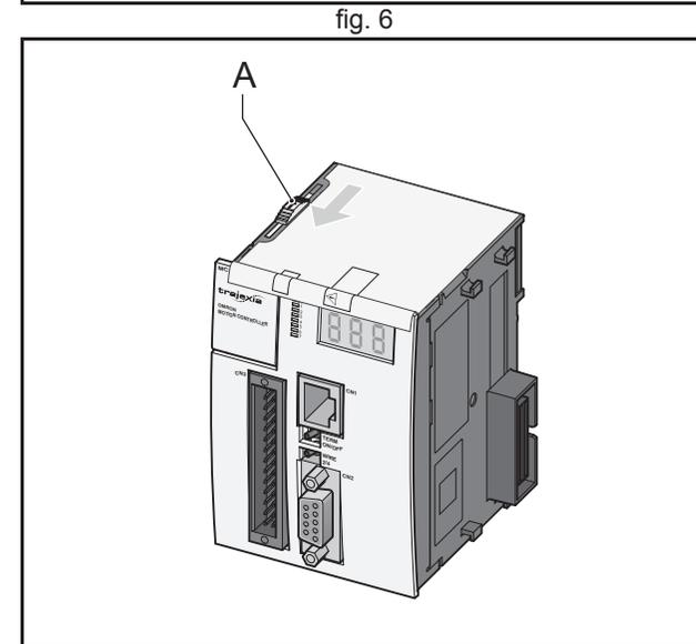
6. Attach the TJ2-MC\_\_ (C) to the Power Supply Unit (B).
