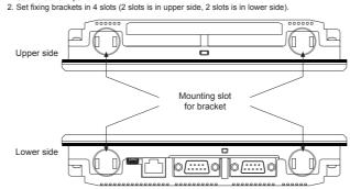
Tighten fixing bracket with M4 screw driver and tightening torque is 0.3 to 0.5Nm.
