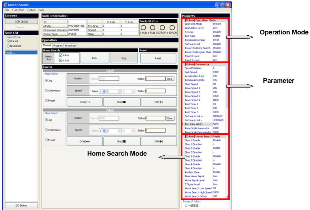
[Operation Mode], [Parameter] and [Home Search Mode] are in the [Property]section on the right side of the screen. Y axis properties are under the X axis properties.
