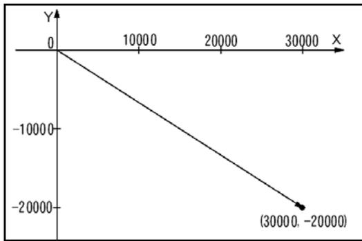
The above image shows motion when the end coordinates are set to (30000, -20000) from the present coordinates (0, 0). The coordinate range of X, Y axes is  $-8,388,608$  to  $+8,388,607$ .
