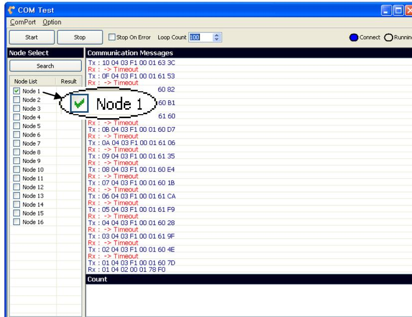
In the above case, only Node 1 is connected to PC.
