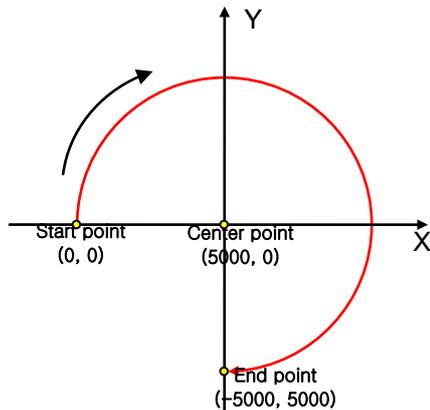
In the above image, center coordinates (5000, 0) and end coordinates (5000, -5000) are set from present coordinates (0, 0) using FID command. The radius of the circle is 5000, and it drives from present coordinates (0, 0) to end coordinates (5000, -5000) in CW direction.
