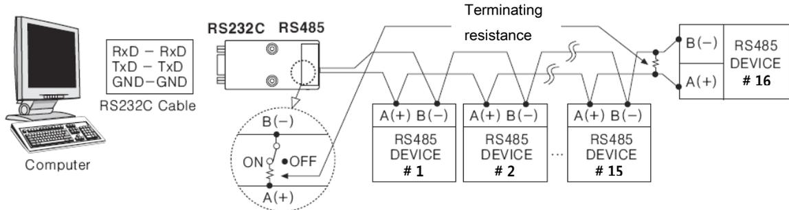
(The connected communication converter is SCM-38I of Autonics.)
