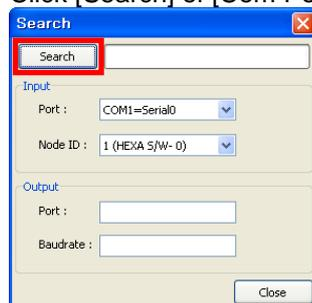
Select [Port] and [Node ID] of [Input] for the connected motion controller. Click [Search] at the top. The Motion Controller's current communication speed is shown in [Baudrate] of [Output].
