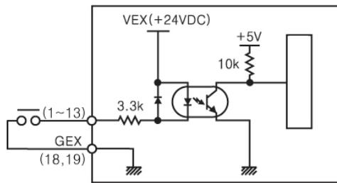
&lt; CN3 control input signal circuit &gt;
