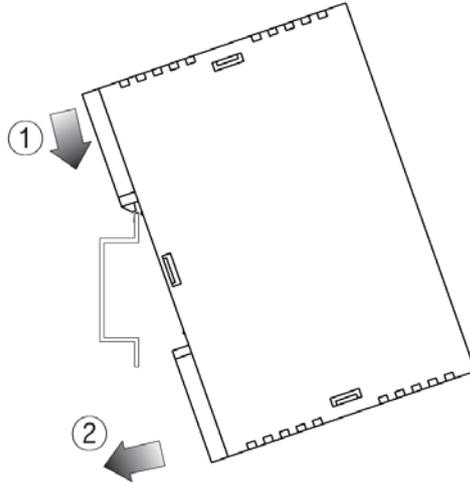
2nd Engage the top and bottom rail locks. Push until it clicks and the rail locks firmly fix the DIN rail.
