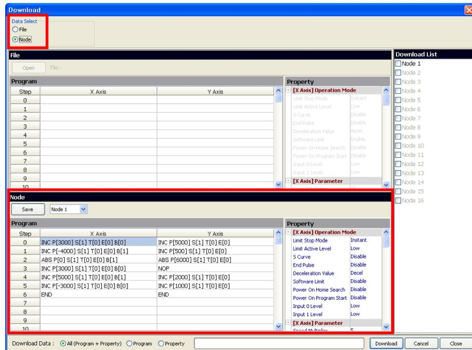
2nd Select the number of node to download in [Node] section. Only communicating nodes are activated.
