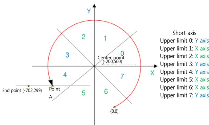
In the above image, center coordinates (-200, 500) and end coordinates (-702, 299) are set from present coordinates (0, 0) using RID command. It starts drive in CCW direction with the radius defined by present and center coordinates. The specified end coordinates are on upper limit 4. Therefore the Y axis is the short axis. When the Y axis value of the end coordinate reaches 299, it is considered the end of interpolation.
