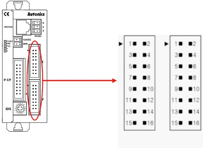
※ CN4, CN5 connector deployments of PMC-2HSP/2HSN-USBAre the same as for PMC-2HSP /2HSN-485 model.
