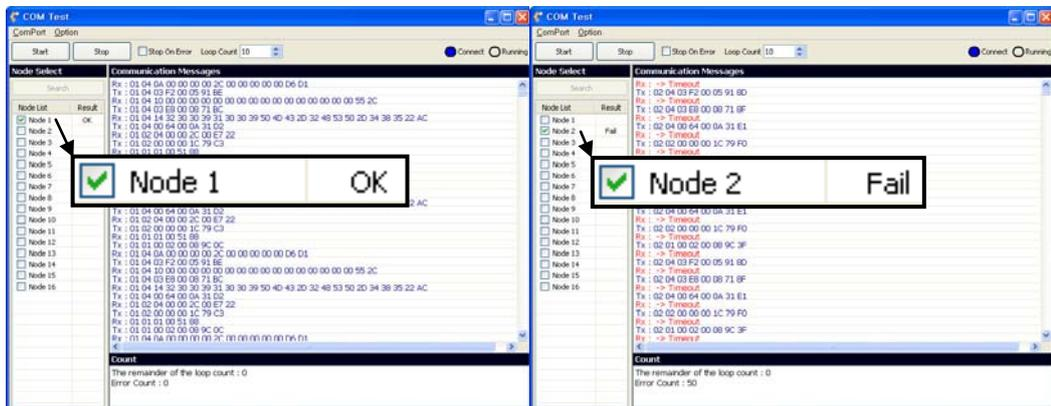
When the test has started, Rx and Tx communications messages are displayed for successful connections and unsuccessful connections. When the test finishes, [Result] box in [Select Node] section displays the test result (OK/Fail). If the communications failure happens repeatedly, inspect communications environment again.
