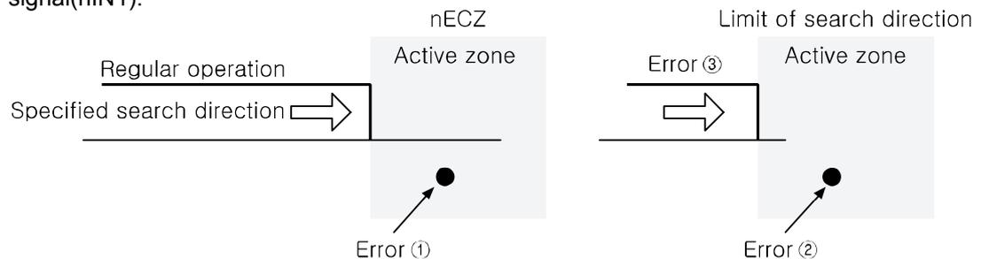
When encoder Z-phase signal(nECZ) is active, it clears actual position counter(EP). Refer to the Actual position counter clear by external signal '5.3.4 Actual position counter clear by external signal'.
