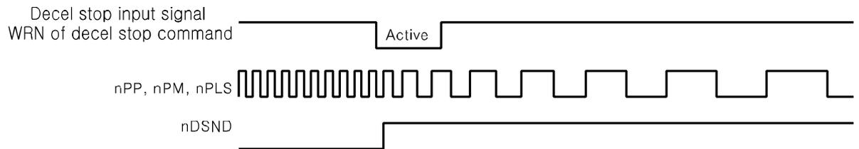
When as input signal filter is set as valid, input signal is delayed filter pass time.
