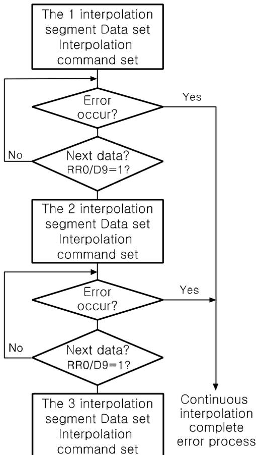
In consecutive interpolation, use D9(CNEXT) bit of RR0 register. This bit is the data of the next interpolation node and it is the whether to set interpolation drive command during interpolation drive. '1' means set available and '0' means set unavailable.
