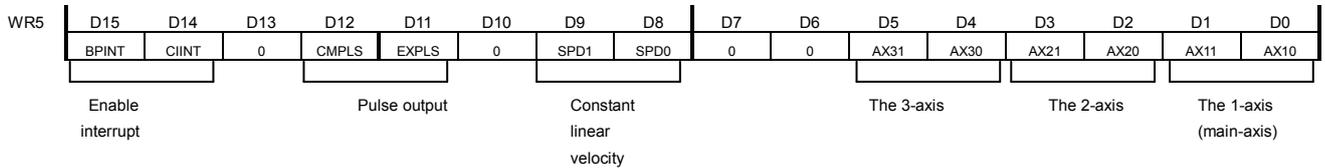
D1, 0      AX11, 10      Designate the 1-axis (main-axis) to execute interpolation drive. Refer to below table for axis code.
