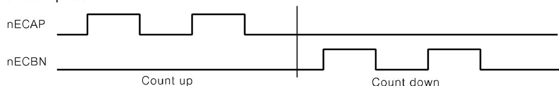
Select the pulse input method by D9(PINMD) bit of WR2 register and encoder 2-phase pulse input divided ratio by D11, D10(PIND1, 0) bit.
