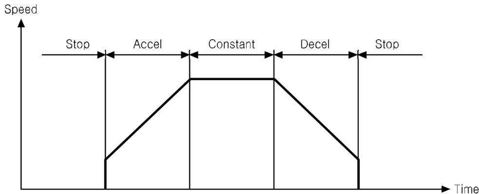
In each axis drive, the acceleration/constant speed/deceleration status of drive speed outputs at D2(ASND), D3(CNST), D4(DSND) bit of RR1 register for each axis and at nOUT6/ASND, nOUT7/DSND signal. Because signal output is used with general output signal terminal, to output drive status, set D7(OUTSL) bit of WR3 register as '1'.
