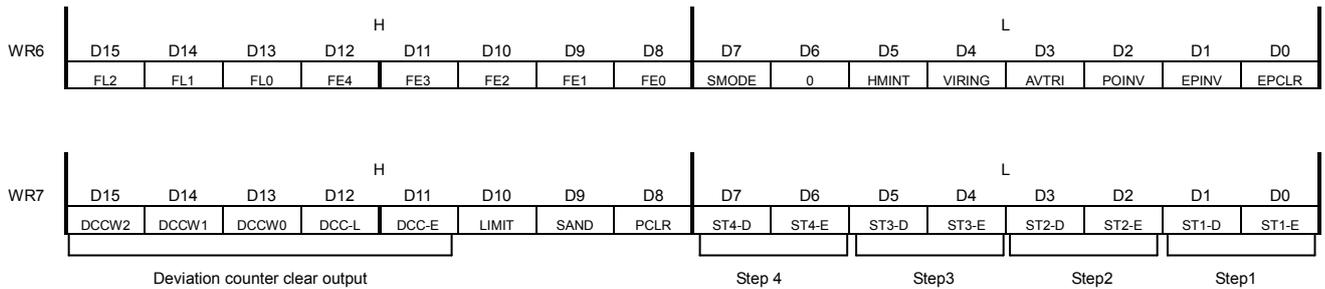
WR6/D0      EPCLR      When drive stops by nIN2 signal, it clears actual position counter. When setting this bit as '1' and nIN2 signal is changed active level during driving, drive stops and actual position counter(EP) is cleared. Set WR1/D5 (IN2-E) bit as '1' and WR1/D4(IN2-L) bit as valid level. Refer to '7.4 WR1 mode register 1'.
