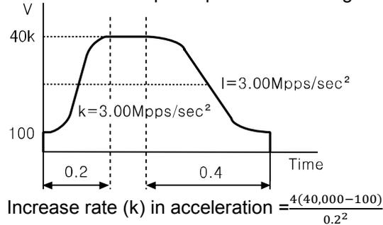
$$\text{Increase rate (k) in acceleration} = \frac{4(40,000-100)}{0.2^2} = 3.99\text{Mpps/sec}^2$$
