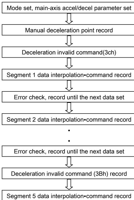
Be sure that manual deceleration point is the value for the number of main axis basic pulses from node 5. For example, deceleration pulse is used 2000, the number of basic pulses which is output to node 5 is 5000. Set manual deceleration point as  $5000-2000=3000$ . From starting deceleration to stopping, it must be set in one node. In other words, deceleration stop's last node requires that the total number of used output pulses should be over the number of the pulses for deceleration.
