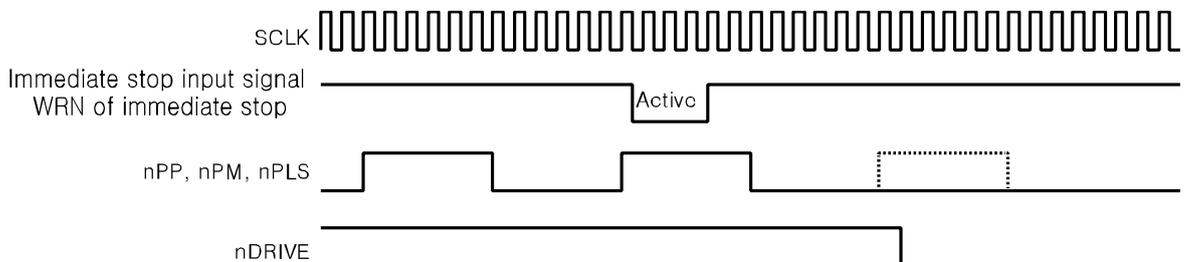
Immediate stop input signal requires pulse width over than CLK2 cycle even though input signal filter is invalid. When input signal filter is set as valid, input signal is delayed by filter pass time.
