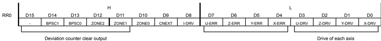
Be sure that D7 to D4(n-ERR) bit for each axis' error may indicate '1' even though the normal operation of limit signal due to irregular operation of Step 1, 2. This error bit should be checked when auto home search completes not during auto home search running.
