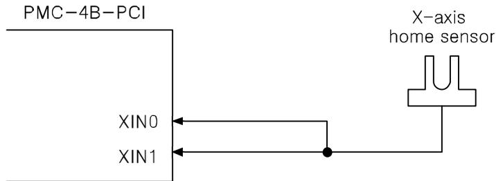
As the above table, set signal logic level of Step1 and Step2 as search direction as same. (It is possible to set logic level as reverse.) When home searching at Step1 with high speed and home signal becomes active, it stops by deceleration.
