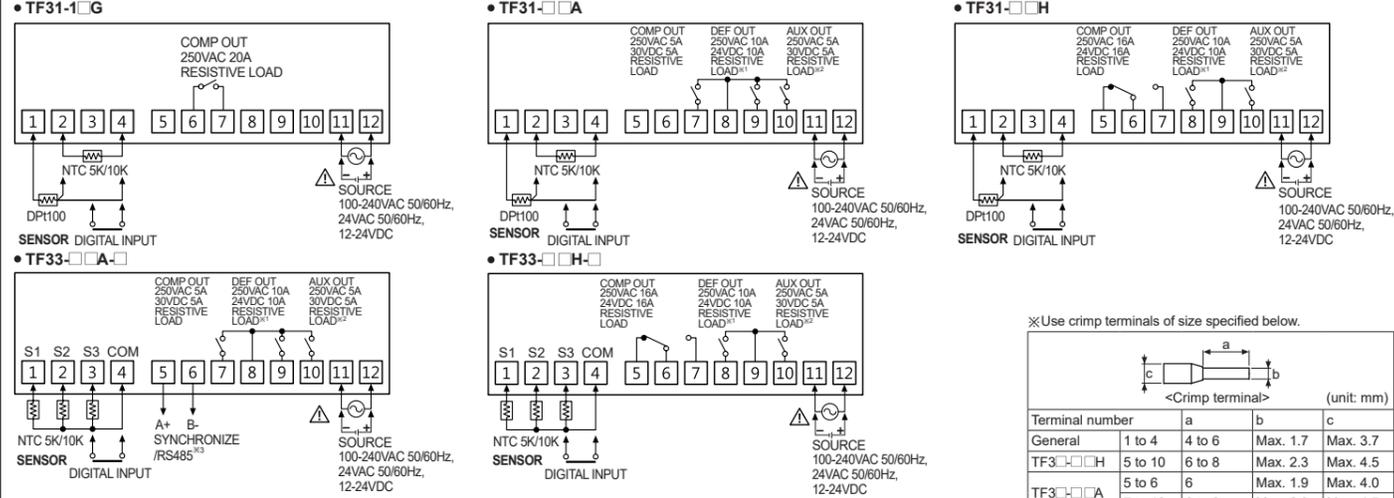
※1: Only for compressor+defrost or auxiliary (alarm/evaporator-fan) output model (TF31-1-G), compressor+defrost+auxiliary (alarm/evaporator-fan) output model (TF33-3□□□□).
