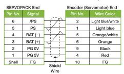
Note: The signals BAT(+) and BAT(-) are used when using an absolute encoder.
