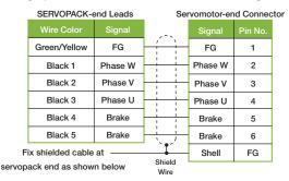
Note: No polarity for connection to a holding brake.
