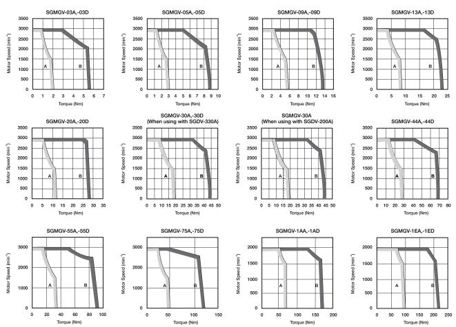
Notes: 1 When the effective torque during intermittent duty is within the rated torque, the servomotor can be used within the intermittent duty zone.
