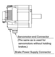
**Brake Power Supply Connector** 0.85 to 15 kW
