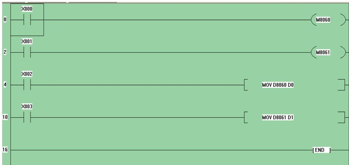
**Note:** When M8060 or M8061 is edited in the PLC program, the original function of HDI with P.550 set to 54 in SA3 and SF3 becomes invalid when PLC is valid, and the original function of M2 terminal with P.82 set to 54 in SE3 becomes invalid.
