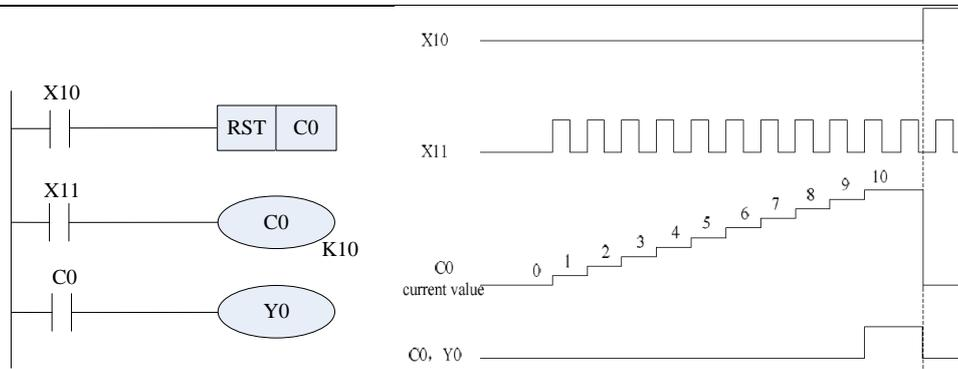
As shown in the figure above, the current value of C0 will increase by 1 once X11 ON->OFF. When the count value reaches K10, the C0 contact will act and Y0 will be output. After X1 triggers C0 again, it will not accumulate and stay at K10. When the power supply is normal, the current value register of the counter has a memory function, so the RST reset instruction must be used to reset the current value register before the counter restarts counting.
